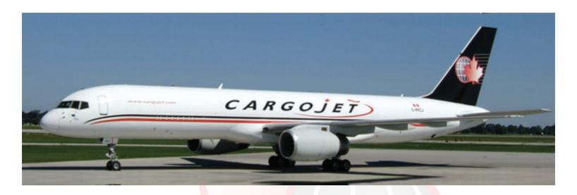
Cargojet's state of the art B757-200ER freighter is capable of carrying a structural payload of up to 80,000 lbs utilizing 15 upper deck positions and loose load lower hold cargo compartments.
