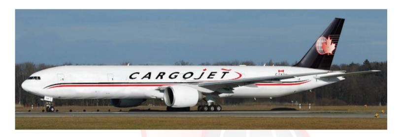
Cargojet's state of the art fleet of B777-300ERSF freighters are capable of carrying a structural payload of up to 222,000 lbs utilizing 33 main deck positions, and 14 lower deck positions with 600 cubic feet of bulk cargo hold area.
