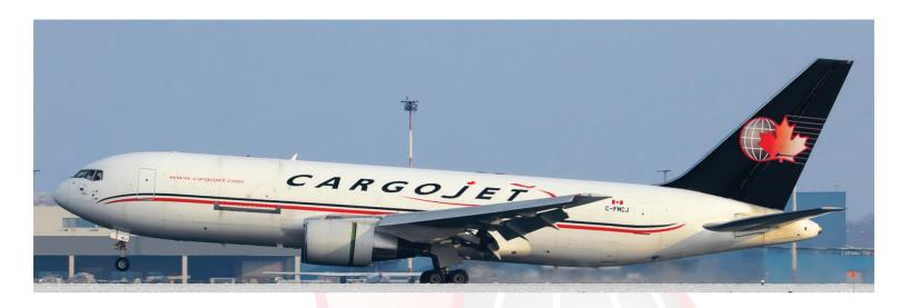
Cargojet's state of the art fleet of B767-200ER freighters are capable of carrying a structural payload of up to 100,000 lb utilizing 19 upper deck positions, containerized (LD8 & LD2) and loose load lower cargo hold compartments.
